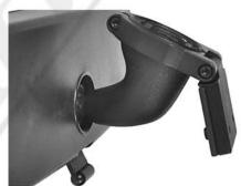
5 - Reattach right side of the mount. Make sure small lock washer is still on lower screw and tighten until fairly snug. Leave top screw loose so mount can slide towards windshield around the large diameter of the mirror stem. Slide the mount upwards leaving approximately 1/8" of clearance between mount and the windshield. Rotate mount until level from side to side and tighten the top screw.
