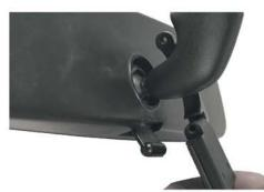
4 - Install mount from passenger side of the vehicle. Remove right half of the mount by removing the two socket head cap screws. Be aware there is a small lock washer on the lower screw. With left half of the mount still attached, position the mount around the mirror stem as shown above.
